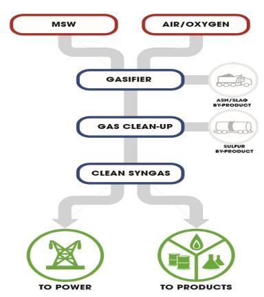
What's produced is a synthesis gas (syngas) that can be converted into electricity and valuable products. With gasification, MSW and wastes are no longer useless, but they become feedstocks for a gasifier. Instead of paying to dispose of and manage the waste for years in a landfill, using it as a feedstock for gasification reduces disposal costs and landfill space, and converts those wastes into valuable electricity, fuels, chemicals or fertilizers.
