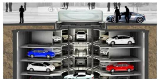
A robotic parking system reduces the space needed for cars by 50% and creates more space for design, development and the community. The speed and
